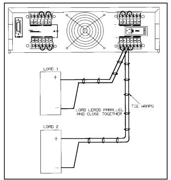
Figure 4-4. Optimum Hookup for Multiple Loads, Local Sensing
